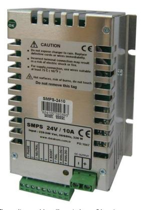
The units provide a "boost charge" input as a standard feature. When this input is pulled to battery negative, the output voltage of the charger will be set to the boost charge voltage. This feature may be used temporarily to improve battery life.
