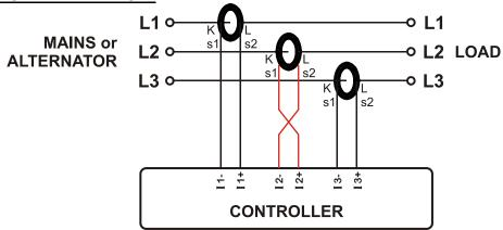
The generator is still loaded with 100 kW On each phase. The load Power Factor (PF) is 1. PF in phase L2 will show -1,00 due to reverse CT polarity. The result is that total generator power displayed by the controller is 100 kW.
