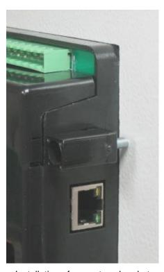
Installation of screw type bracket
