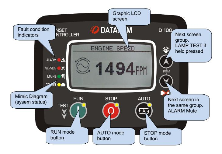
When the engine hours <u>OR</u> the time limit is over, the **SERVICE REQUEST** led (red) will start to flash and the service request output function will be active. The service request can also create a fault condition of any level following parameter setting.
