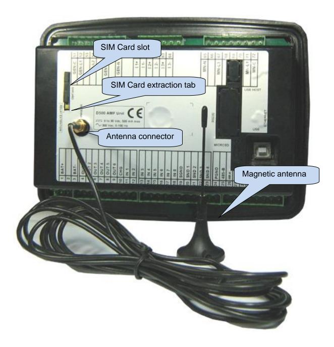
The module requires a GPRS enabled SIM card for full functionality. Voice-only type SIM cards will usually not function properly.
