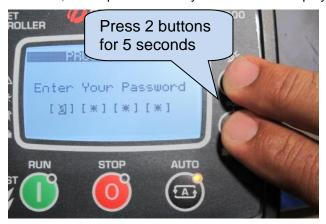
A 4 digit password must be entered using **(a) (b) (b)** buttons.
