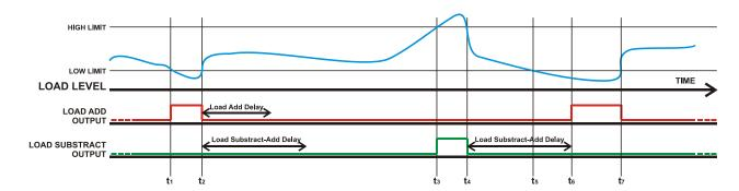
t1: the load goes below the Load Shedding Low Limit, thus the Load Add output becomes active.
