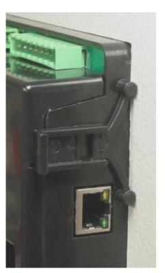
Installation of self retaining type bracket
