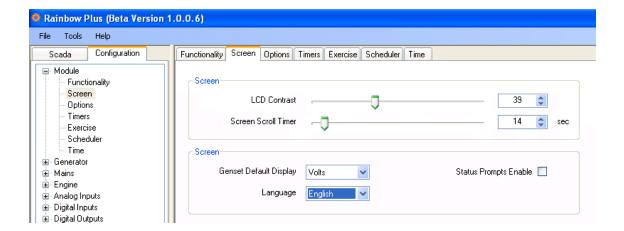
Eventually the same parameter can be modified through the front panel programming menu. The related parameter is Controller **Configuration > Screen Scroll Timer**.
