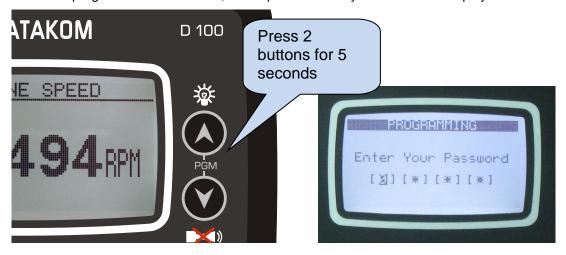
Skip the password entry screen by pressing the button 4 times. The screen below left will come.
