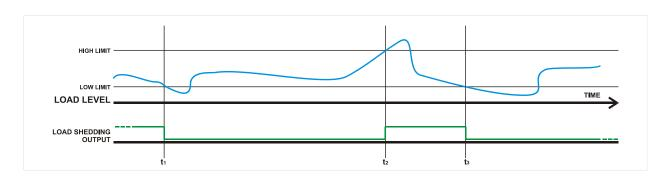
t1: the load goes below the Load Shedding Low Limit, thus the Load Shedding output becomes inactive.
