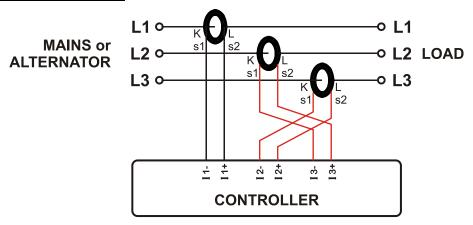
The generator is still loaded with 100 kW on each phase. The load Power Factor (PF) is 1. PF in phases L2 and L3 will show -0,50 due to phase shift between voltages and currents which is caused by CT swapping. The result is that total generator power displayed by controller is 0 kW. Measured values are as follows:
