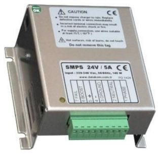
The units provide a "boost charge" input as a standard feature. When this input is pulled to battery negative, the output voltage of the charger will be set to the boost charge voltage. This feature may be used temporarily to improve battery life.
